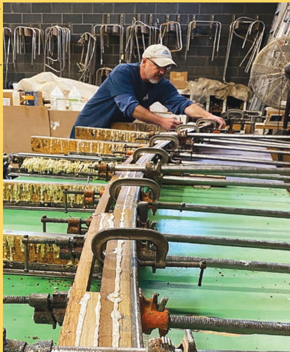
The first teak slats are glued and held in place with 3-inch stainless steel screws. Slats and blocks are put in place until this transom platform, for a 46-foot Grand Banks yacht, reaches 25 inches deep.
