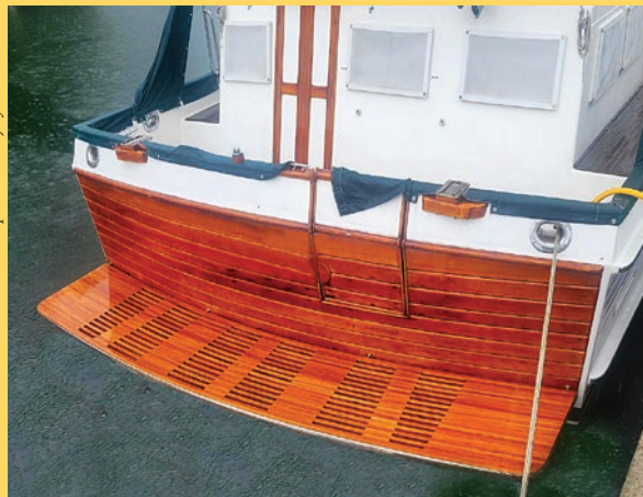
The final teak transom platform built by Butler Marine Products, Luzerne County, matches the original wood of this 46-foot Grand Banks.
